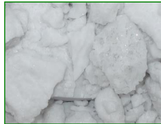
FLiBe molten salt (left: 1kg; right: 10 kg)
