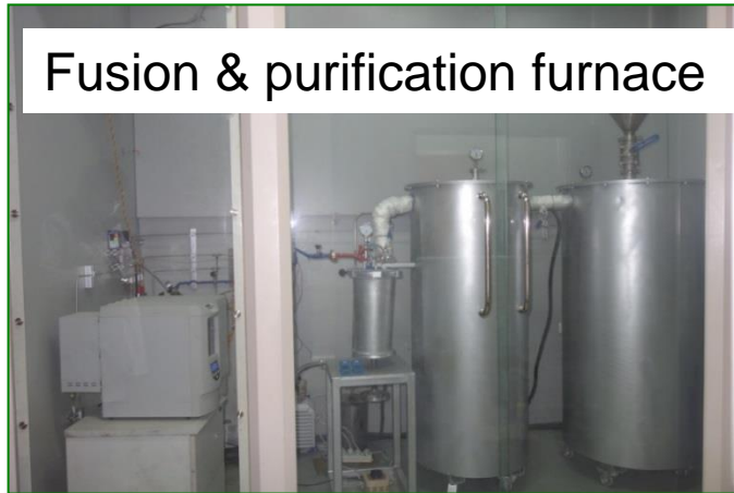
Equipment for the preparation of FLiBe (10kg scale)
