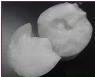
FLiBe molten salt (left: 1kg; right: 10 kg)
