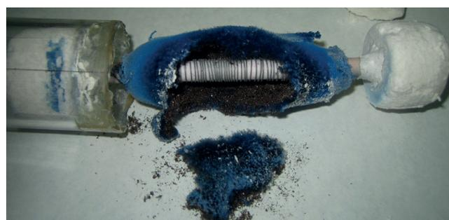
Fig. 14. Reactor KV3 opened after ending of experiment.
