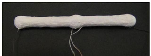
**Fig. 4.** The scheme of Rossi's reactor analogue [26]: 1 – cement, 2 – electric heater, 3 – ceramic bungs, 4 – ceramic tube, 5 – thermocouple, 6 – powder of  $\text{Ni} + \text{LiAlH}_4$ . Below – foreign view.
