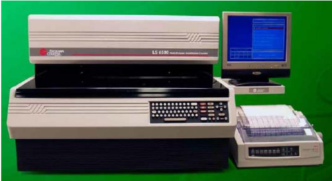
Figure 2.3-5. Photograph of the Beckman Coulter LS6500 multipurpose scintillation counter.
