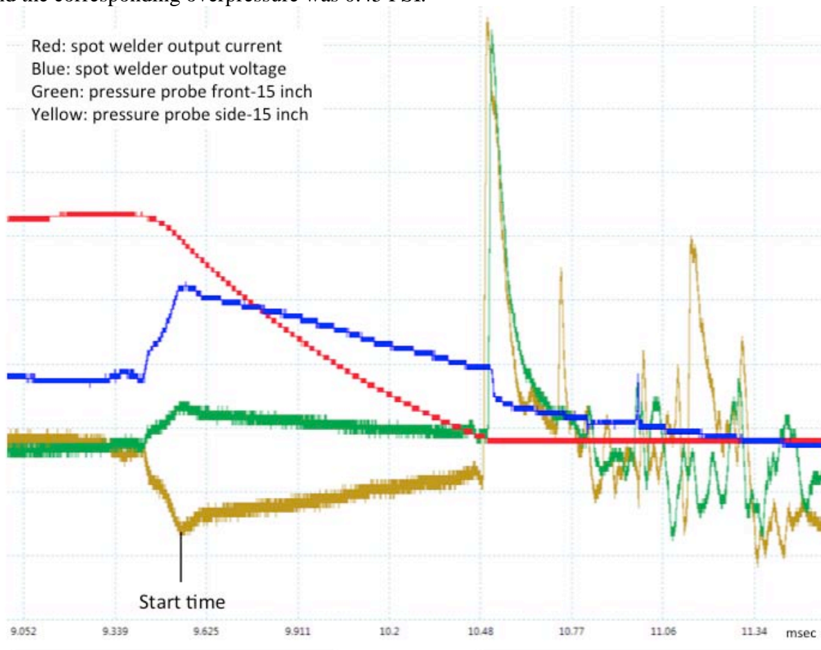
Figure 55. Welder trigger and pressure sensor data for sample Ti powder ( 15 \text{ mg}/3.1 \times 10^{-4} \text{ moles} ) + \text{H}_2\text{O} ( 5 \text{ mg}/2.8 \times 10^{-4} \text{ moles} ) in the Al DSC pan as a function of time showing the detonation shockwave that is faster than sound speed. A later reflected peak is also observed. The EMP spike was used as the start time of the shockwave. The shockwave speed was 400 \text{ m/s} and the corresponding overpressure was 0.45 \text{ PSI} .
